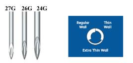
Needle gauge corresponds to the outer diameter of the needle. Given a specific needle gauge, the inner diameter is determined by the wall thickness of the needle. In general, a thinner wall (i.e. larger inner diameter) may present less insertion force as well as a lower resistance to the flow of medication. A thinner wall may make the needle less robust and thus increase their proneness to damage during insertion or handling.
